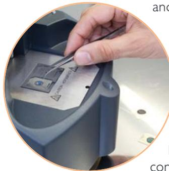
At the end of the measurement the plastic sample is discarded and the built-in software calculates and stores all relevant information. A certificate of OIT conformance can be printed and used as part of your, or your customer's, quality control process.
